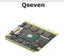
Intel-based: several CPU 's Standard Size (70 mm x 70 mm)
